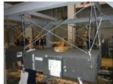
Test of heavy equipment holder
