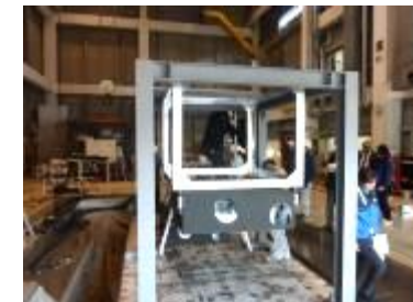
ECO support bracket seismic test
